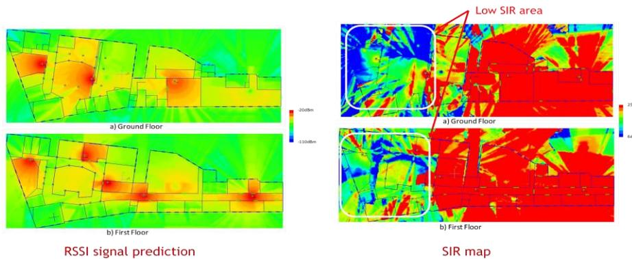
Figure 2: Downlink system-level simulation when using closed access
