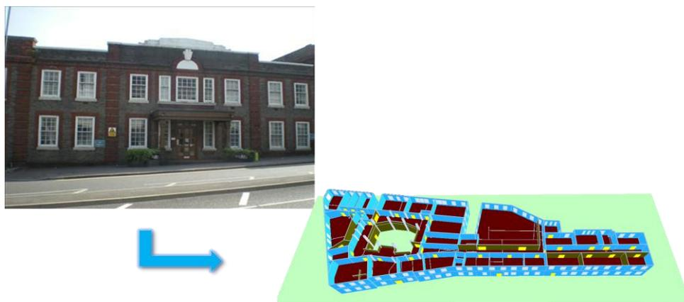
Figure 3: screenshot from iBuildNet providing a 3D view of coverage simulation in a building
