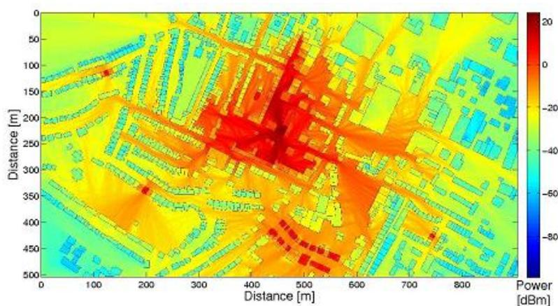
Figure 5. Best-server coverage in a hybrid macro-femtocell scenario with a densely deployed street and some randomly located femtocells
