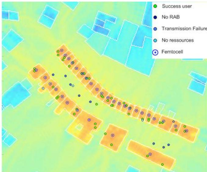
Fig. 7. Downlink system-level simulation when using closed access
