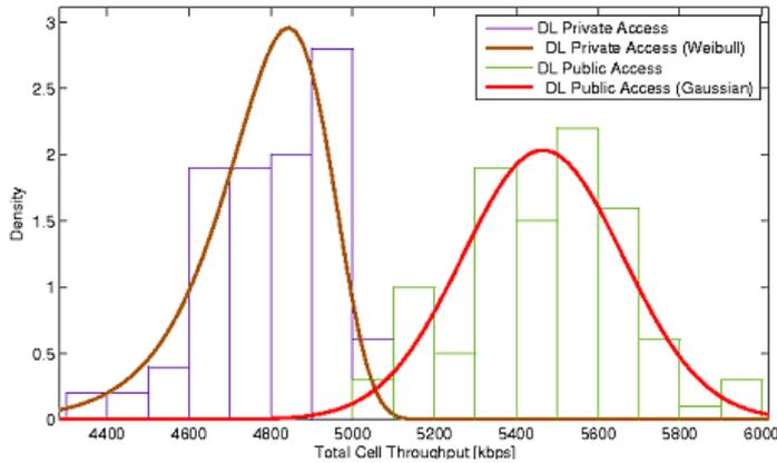
Fig. 8. Downlink total cell throughput PDF
