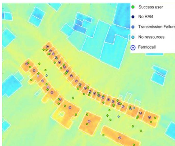
Figure 6. Downlink system-level simulation when using open access
