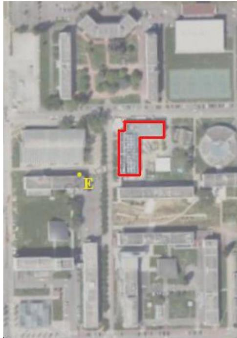
**Figure 3.5: outdoor to indoor scenario.** In red: the building where the indoor measurements were performed. E1 and E2 represent the position of each emitter and the black arrows show the directions where the directive antennas were pointing.
